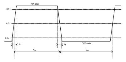
Picture 3.2 Waveform of the optical test output
