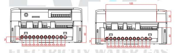
Figure 2.3 Meter terminal dimensions (with GPRS modem left, witout modem right)
