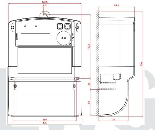
Figure 2.2. Dimensions of the meter
