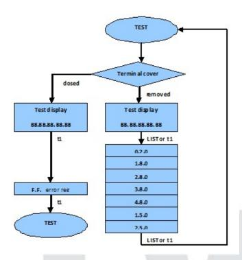
Figure 4.4 Display navigation diagram – test mode
