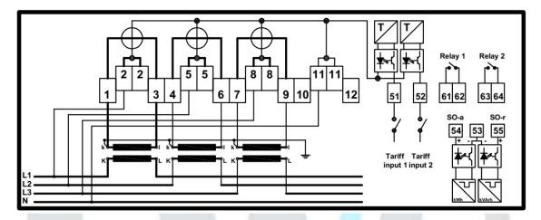
**Figure 2.7** Current transformer operated meter connection scheme
