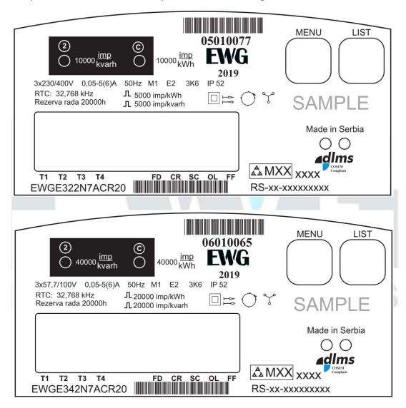
Figure 2.5 Name plates of E32xxx and E34xxx meters
