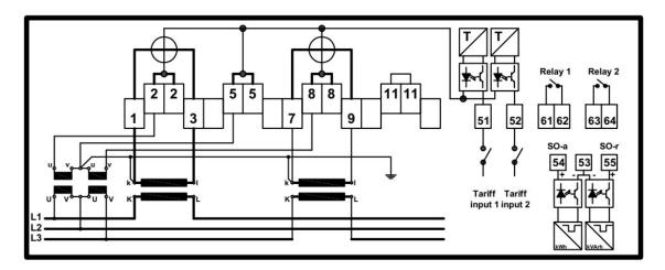
Figure 2.9 Current and voltage transformer operated meter Aaron connection scheme
