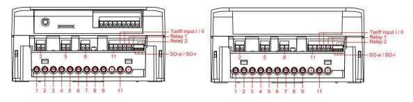
**Figure 2.4** Meter terminal connector's labels (with GPRS modem left, witout modem right)
