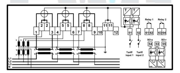
Figure 2.8 Current and voltage transformer operated meter connection scheme
